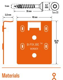
B-Fix Border: 301 stainless steel B-Vis Border: A2 stainless steel + silver coating
